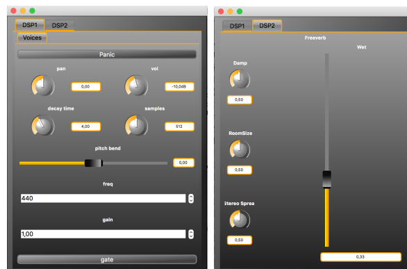
Figure 5: Polyphonic instrument with output effect GUI interface: left tab window shows the polyphonic instrument with its Voices group only, right tab window shows the output effect.
