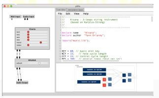
*pMix is written using C++ and the JUCE framework.* In order to integrate FAUST's LLVM compiler, a JUCE module was developed so that other JUCE users can also easily integrate FAUST into their projects.
